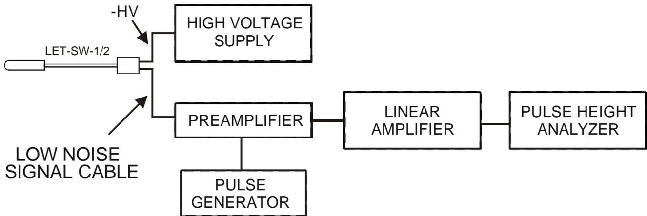
Figure 2 Electrical Interconnection Diagram for LET-1/2 Operation
