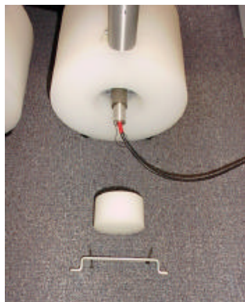
Picture of the detector after removal from the moderator.
